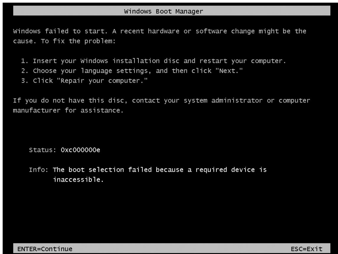
FIGURE 13-10 Windows Boot Manager after trying to load a disk with an orphaned disk signature.
