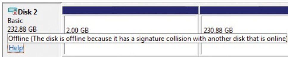
FIGURE 13-8 Disk Management shows a signature collision preventing a disk from being brought online.
