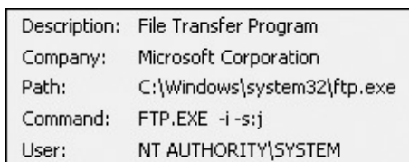
FIGURE 20-83 FTP.EXE launched with command line -i -s:j .
